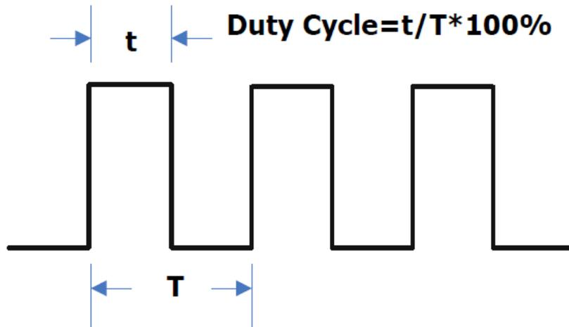
The setting range of duty cycle is limited by the “FREQ” setting. Please refer to “**Waveform Characteristics**” in “**Specifications**”. The default value is 50%.
