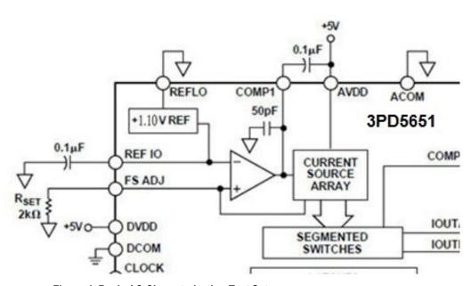
Figure 4. Basic AC Characterization Test Setup
