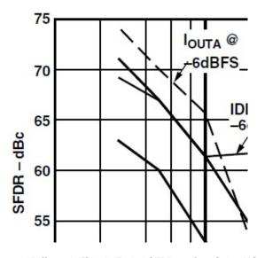
Figure 8. Differential/Single Ended SFDR vs. fout @ 100 MSPS
