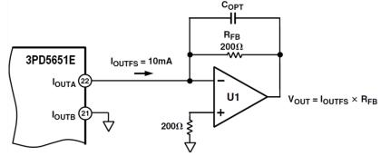
Figure 17. Unipolar Buffered Voltage Output
