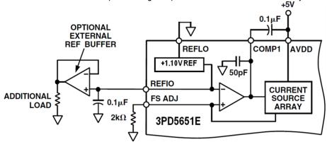
Figure 14. Internal Reference Configuration
