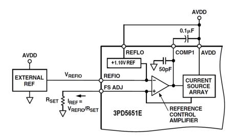
Figure 15. External Reference Configuration
